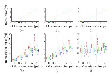
Fig. 2: *Image noise experiment*. Methods BA, SO, and ASO in red, green, and blue, respectively, on calibration and validation data point sets. (a–b) barrel distortion, (c–d) pincushion distortion (e–f) zero-crossing problem.
