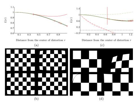
Fig. 1: *Calibration issues*. Examples of issues arising while using polynomial and rational function for radial distortion calibration. See text for details.
